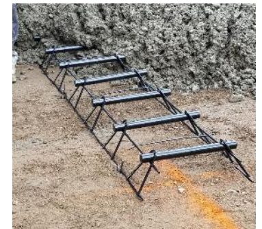
Carbon Steel with A934 Epoxy and Abrasion Resistant Overcoat Approved 2017*
