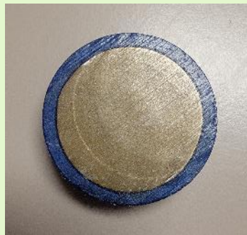
Glass Fiber Reinforced Dowel over Carbon Steel Bar Approved 2013
