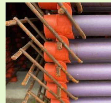
Zinc Galvanized Tube with A934 Epoxy Approved 2016*
