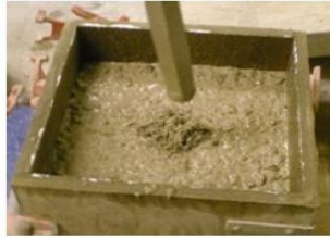
Figure 3 —Box Test Steps (Cook et al., 2015) (Source: Oklahoma Transportation Center)
