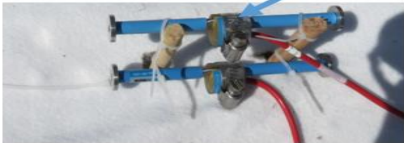
Vibrating wire (VW) strain gauges (odd # Top and Even # Bottom)
