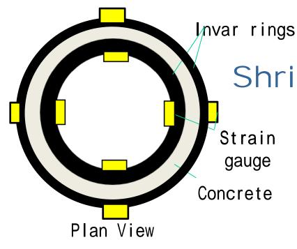
Shrinkage: Dual Ring Test
